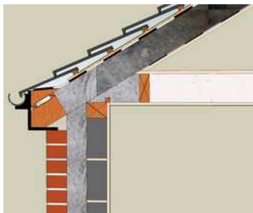
Detailing for eaves using insulation between rafters
